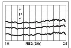
Center trace is phase response of 8491A -6 dB attenuator from 1.0 to 2.0 GHz taken with the 8410 network analyzer. Top and bottom traces are  $\pm 1^{\circ}$  calibration. Linear phase component has been compensated for with a line stretcher. Response, therefore, shows nonlinear phase deviation of  $< \pm \frac{1}{2}^{\circ}$  over 1 to 2 GHz band.
